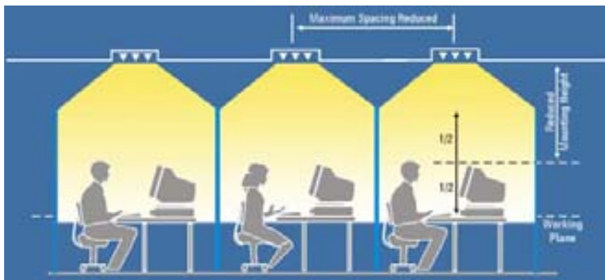
Adjusted spacing criterion and mounting height to accommodate partitions.
