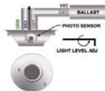
Figure 9.11.3. Photosensor and fluorescent dimming ballast for continuous daylight dimming.
