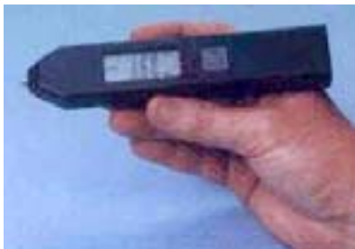
Examples of typical hand-held vibration sensing meters. Note readout providing immediate level indication.
