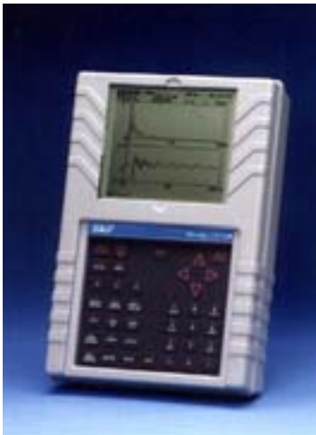
Typical Vibration Analyzer – Note liquid crystal display providing actual vibration waveform information in addition to machine condition analytical capabilities.
